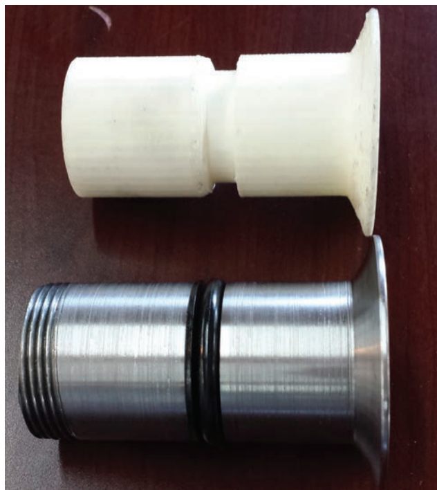
By leveraging the TAZ 3D printer to produce prototype parts in lieu of an outside machine shop, Lightning Hybrids has greatly reduced its development time. Image courtesy of Lightning Hybrids.
