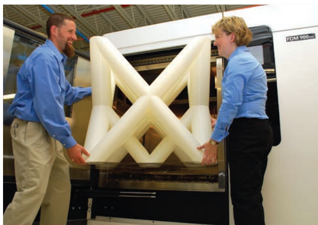
Large FDM machines (such as Stratasys' Fortus 900mc) allow companies to produce parts as large as 36x24x36 in. with real production-grade thermoplastics, making them durable enough for end-use.
